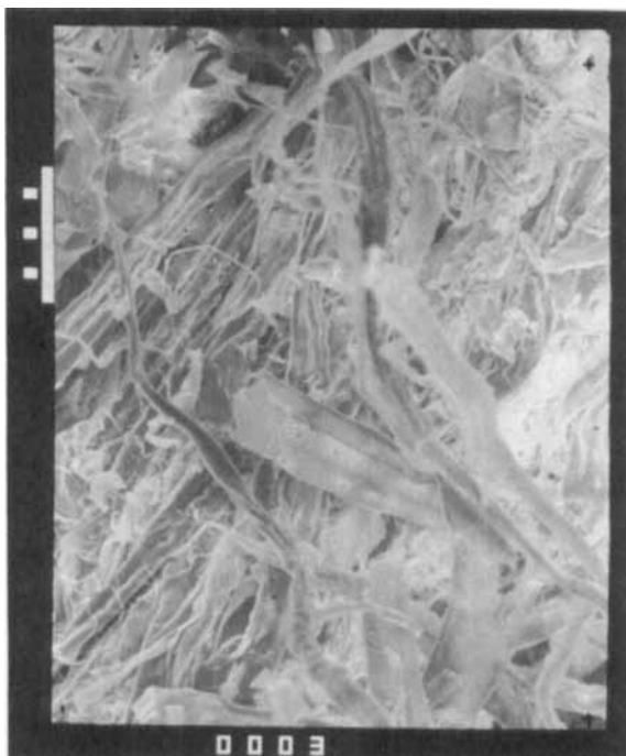
Fig. 1 Scanning electron micrography of: a) the untreated CTMP control (sample A) (x 2500), b) H_2O_2 treated CTMP (sample B) (x 4000), c) the 30% CTMP-PMMA grafted sample (sample C) (x 8000), d) the 50% CTMP-PMMA grafted sample (sample D) (x 8000), e) the 60% CTMP-PMMA grafted sample (sample E) (x 6000)
